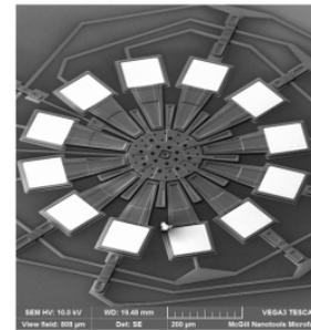
SEM micrograph of micro-motor based MOEMS swept optical elements
