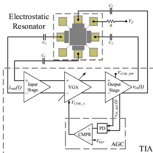
Other MEMS resonator designs based on single wafer technology have also been created by the research team in order to achieve a desirable combination of high quality factor and low motional resistance without requiring any DC voltage for operation.
