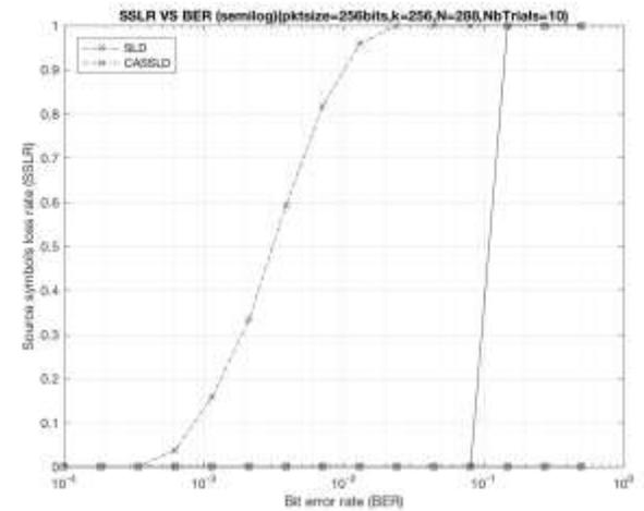
Figure 1: Source symbol loss rate versus bit error rate for various traditional fountain decoding (SLD) and proposed method (CASSLD) for 256 source symbols of 256 bits each and 288 transmitted fountain codes.
